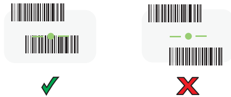
Figure 23 RS6000 Pick List Mode with Multiple Barcodes in Aiming Pattern
