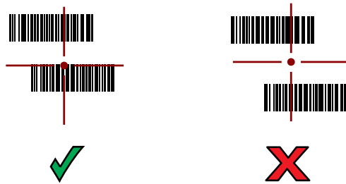
Figure 35 RS6000 Pick List Mode with Multiple Barcodes in Aiming Pattern
