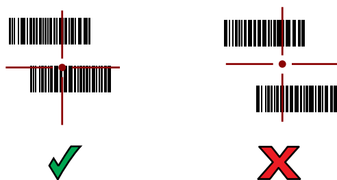
Figure 32 RS5100 Pick List Mode with Multiple Barcodes in Aiming Pattern
