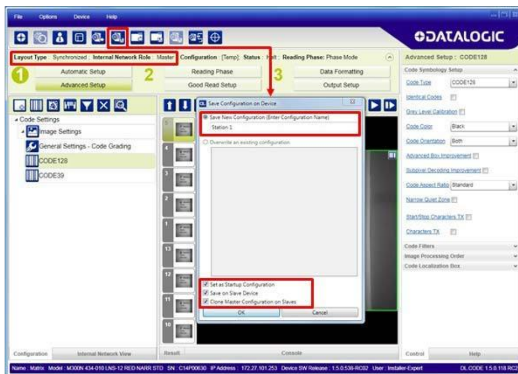
Figure 87 - Saving Synchronized Phase Mode Configuration to Master
