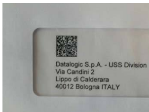
Figure 21 - Address Coded in Data Matrix Symbology for Automated Mail Processing
