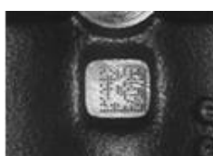
Dot Peening On Scratched Surface
