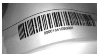
Figure 27 - Barcode Printed on Curved Surface Readable despite Optical Distortion
