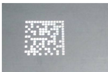
Figure 29 - Dot Peening Marking on Metal Surface with Multi-dot per Code Element
