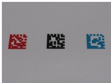
Figure 32 - Data Matrix Codes Printed in Color or on Colored Backgrounds
