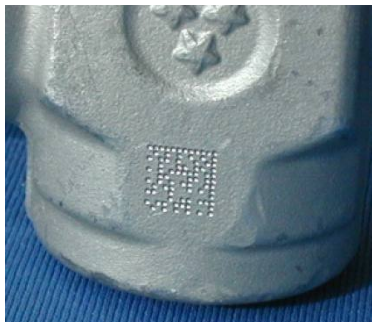
Figure 28 - Dot Matrix Code Directly Marked on Metal Surface by Using Dot Peening Technology
