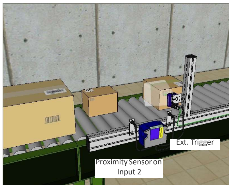
Figure 117 - Example Extending DOF Using External Image Settings Selection
