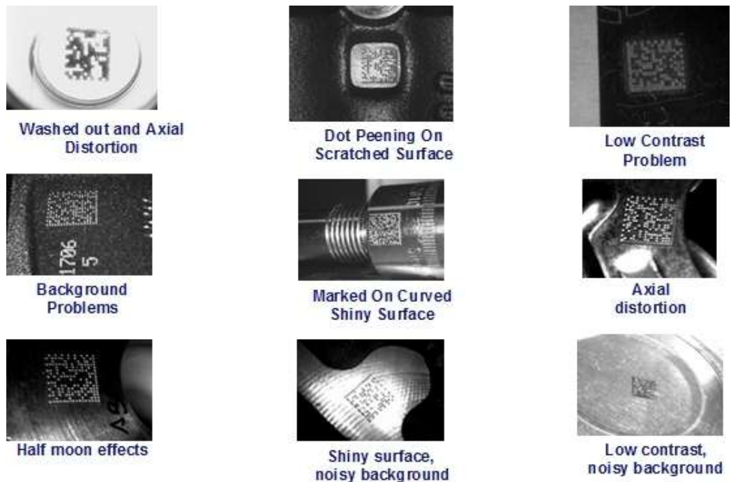
Figure 118 - Problematic Direct Part Marking Examples
